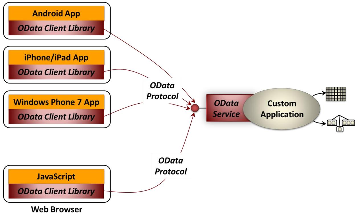
**Figure 3: Mobile phones and Web browsers can use OData to access data exposed by a custom application.**
