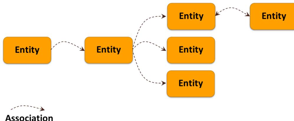
**Figure 6: The Entity Data Model describes data as entities connected by associations.**
